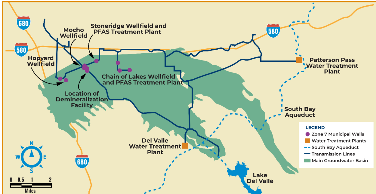
Figure 2. Major Facilities of the Treated Water System
